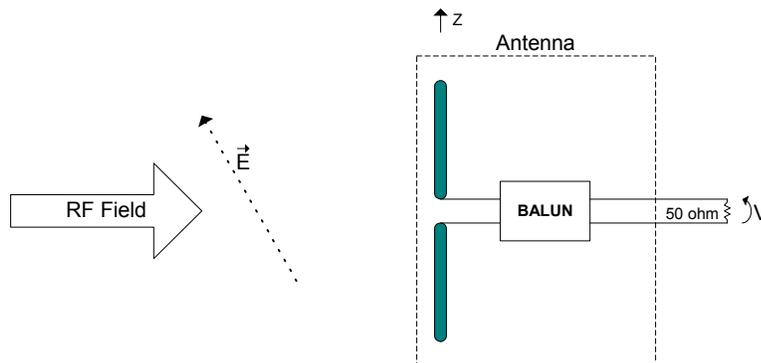
$$\text{Antenna Factor (ratio)} = \frac{|\vec{E} \cdot \vec{z}|}{V}$$
